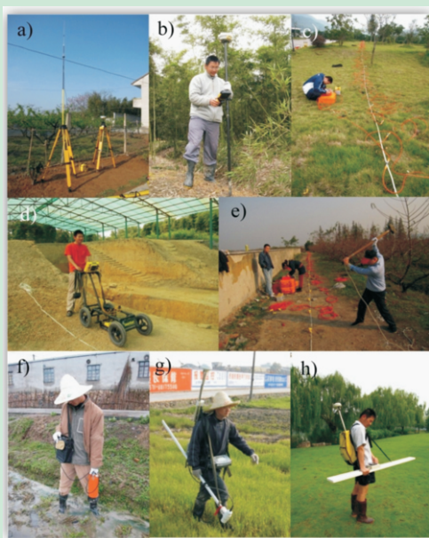
(a) GPS Base Station; (b) GPS Mobile Station; (c) ERT; (d) GPR; (e) Seismic; (f) Radioactive Method; (g) Magnetic; (h) GEM.
